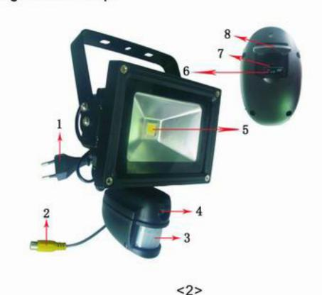
Insert TF card (which with the ".txt" file) into device, connect power, then it will start to record with new modified date&time.
