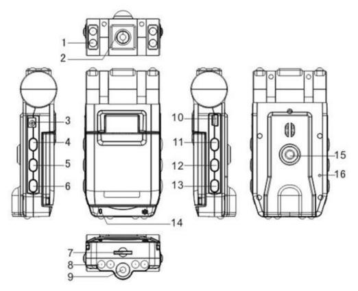
1, Front IR Indicator2,Front Lens3,DC 5V4,ON/OFF5,MENU6,REC/SNAP7,TF8,Rear IR Indicator9,Rear Lens10,USB11,MODE12,UP13,DOWN14,Indicator15,Connection for Mount16,Reset
