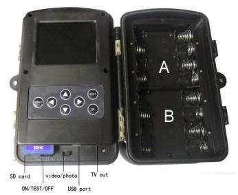
The camera provides the following connections for external devices: USB port, SD card slot, TV out jack, and external DC power in jack .The 3-way Power/Mode Switch is used to select the main operation modes : OFF , ON and TEST.
